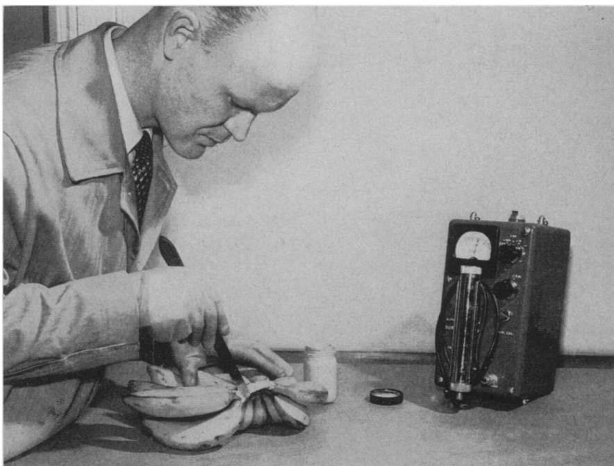
GEIGER CHECK —To prove that a new fungicidal formulation developed to arrest stem rot in bananas does not migrate into the edible portions of the fruit, Dr. John C. McCool, research chemist at the B. F. Goodrich Research Center, uses radioactive tracers.
