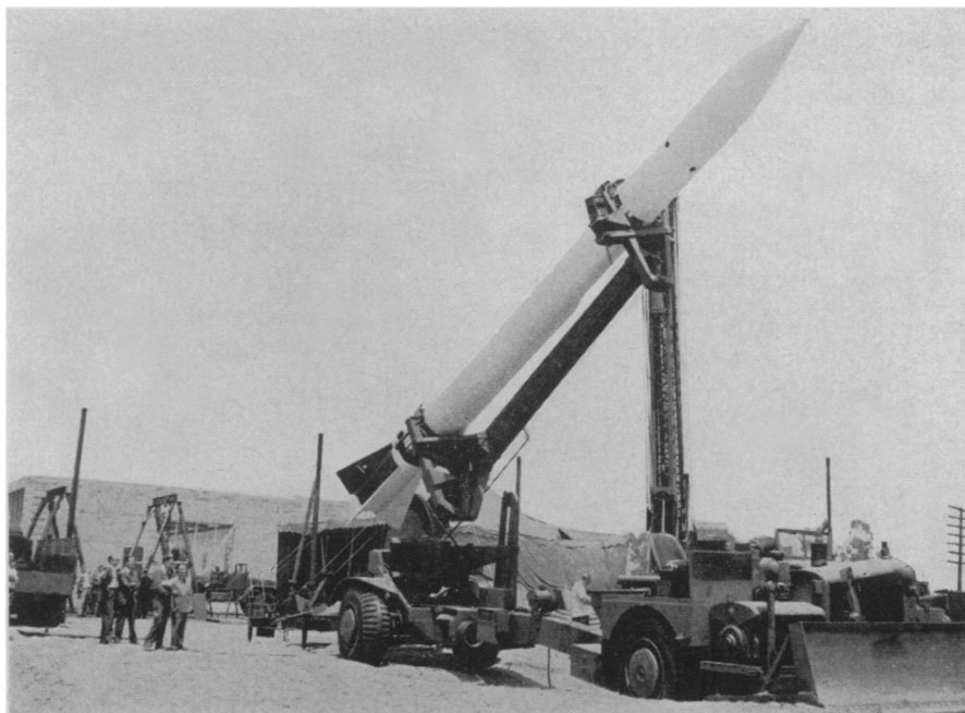
THE CORPORAL —One of the Army's newest guided missiles is this one shown on its launching device. This missile is a surface-to-surface weapon which will carry either atomic or high-explosive warheads and will travel toward its target at several times the speed of sound, propelled by a rocket motor.
