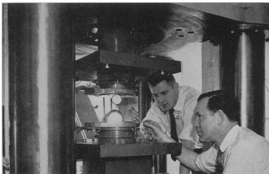
DIAMOND MAKERS —Dr. Herbert Strong (right) and J. E. Cheney watch General Electric's new 1000-ton press, capable of delivering pressures greater than 100,000 atmospheres, or 1,600,000 pounds per square inch, on an area of approximately one square inch.
