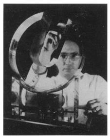
PALOMAR'S "HORSESHOE"—This plastic replica of the two principal bearings that support the 200-inch telescope on Mt. Palomar is shown by Howard N. Kaufman, research engineer for Westinghouse Electric Corporation, which developed the system. A film of oil, three-thousandths of an inch thick, reduces the friction to the point where the huge 500-ton telescope can be moved with a ½-horsepower motor that is only slightly larger than the motor in a washing machine.
