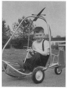
with two-blade, free moving rotor made of tubular steel that forms a "crash protector" for the cockpit. The rudder turns with the steering wheel and the young pilot "flys" his craft with chain-driven foot pedals.
