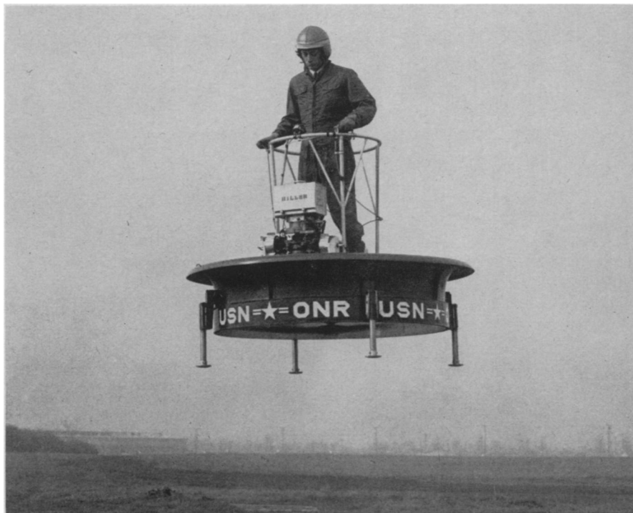
ONE-MAN FLYING PLATFORM —Test pilot Phil Johnston controls horizontal flight of this revolutionary flying machine by merely shifting his weight. Developed by Hiller Helicopters, Palo Alto, Calif., the platform is held in the air by counter-rotating propellers inside the casing.
