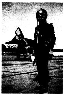
PILOT FASHIONS—The new look for high altitude pilots is this Air Force T-1 pressure suit sported by test pilot Richard L. Johnson. Rubber tubes along the arms and legs inflate, tightening laces that apply pressure evenly over pilot's body.
