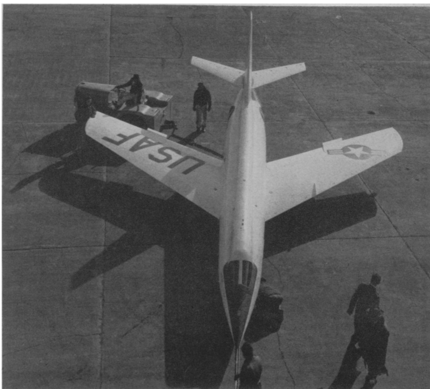
HEAT BARRIER ASSAULT —Designed to exceed the record 1,650 miles an hour set by the Bell X-1A supersonic research airplane, the rocket-powered Bell X-2 is scheduled to begin flight tests soon at Edwards Air Force Base, Calif. Built particularly for heat barrier studies, the sweptwing plane is made of stainless steel to withstand aerodynamic heating and has many new design features.
