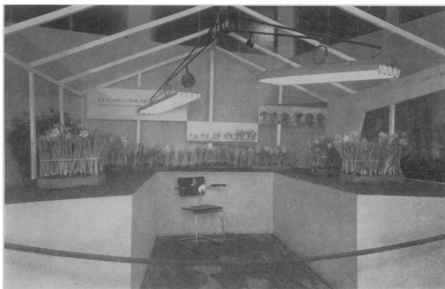
ROTATING HOTHOUSE LIGHTS — To grow hothouse plants more cheaply and efficiently during short winter days, a German scientist, Wilm Kind, devised a method of rotating light bulbs that gives good illumination using only a few bulbs.
