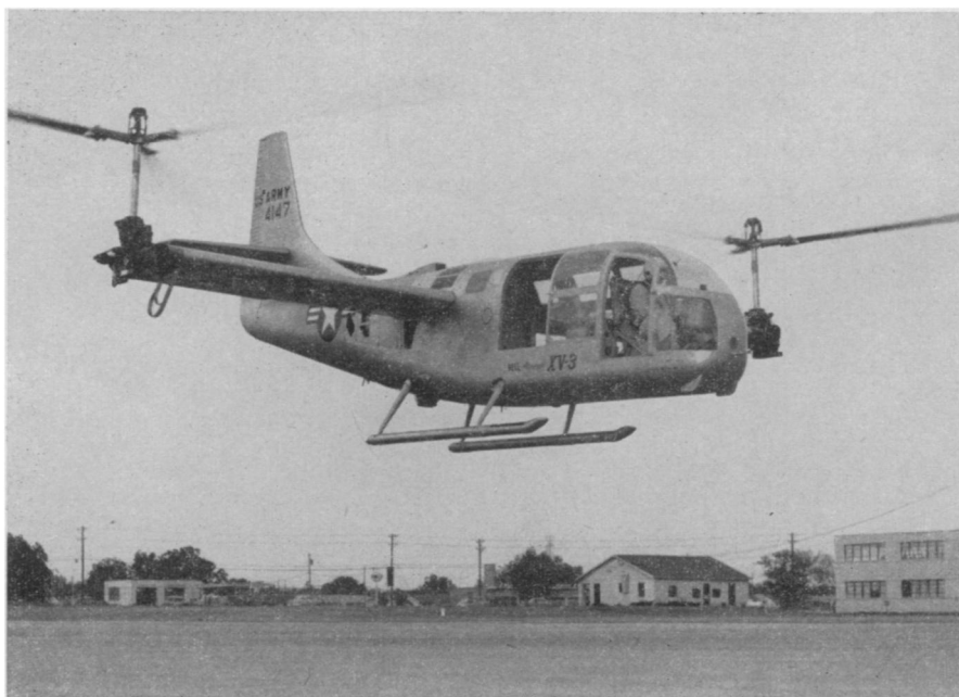
FIRST FLIGHT —The Bell XV-3 convertiplane, developed for the Army, is shown here in its maiden flight. After vertical take-off, the convertiplane was maneuvered as a helicopter. It features combination rotor-propellers that tilt forward from helicopter position to become airplane propellers for long-range, high speed flight.
