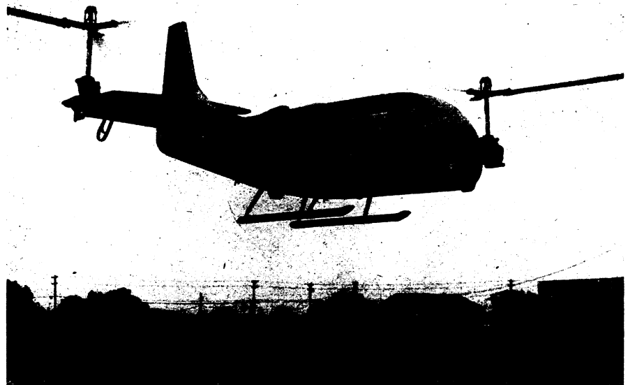
FIRST FLIGHT —The Bell XV-3 convertiplane, developed for the Army, is shown here in its maiden flight. After vertical take-off, the convertiplane was maneuvered as a helicopter. It features combination rotor-propellers that tilt forward from helicopter position to become airplane propellers for long-range, high speed flight.
