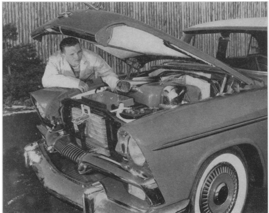
"JET" CAR—A Chrysler Corporation engineer checks under the hood of the firm's experimental "Turbine Special," a 1955 chassis powered by a gas turbine engine. The car is undergoing tests as are gas turbine models designed by other auto manufacturers.
