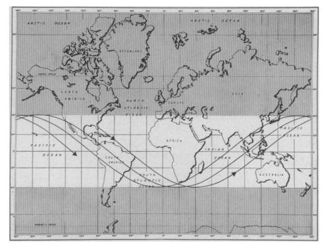
SPOTTING SATELLITE—How the first few revolutions of the satellite through space might appear if its path were projected onto the earth is shown in this diagram. The 25-degree westward displacement after each revolution results from the satellite's elliptical path and the earth's turning. White belt marks limits of visibility on either side of equator.
