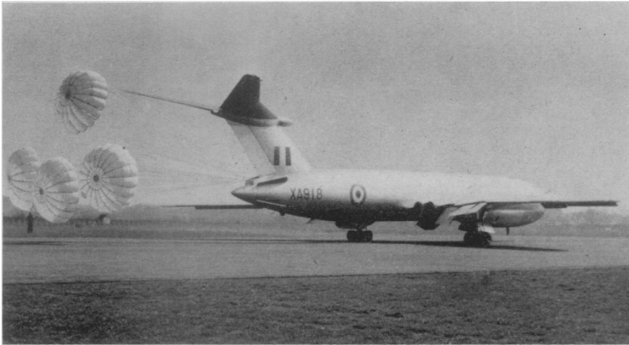
FOUR-PARACHUTE BRAKE —Performance details of this Handley Page Victor jet bomber are still secret but five of them were recently seen in England for the first time by the public. Four parachutes are used to brake the crescent-wing, high-altitude, long-range strategic bomber's landing.
