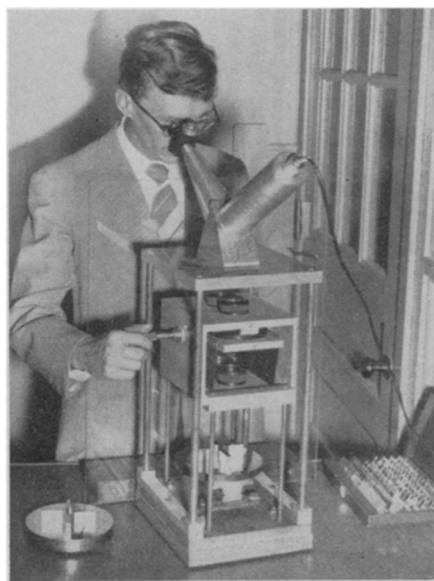
PRECISE DEVICE —This accurate measuring instrument was developed at the National Bureau of Standards for comparing lengths of gage blocks to the nearest ten-millionth of an inch. Theodore R. Young, one of the scientists who designed the device, is shown demonstrating its use.
