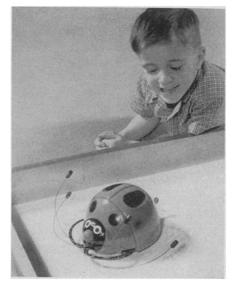
tennae of steel wire activate the steering mechanism. The bug's body is made of an orange acetate plastic.
