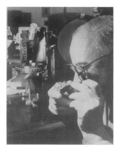
WELDED GRAPHITE—The line between the shiny and dull regions in this piece of graphite, barely visible in the photograph, is the place where two pieces were "welded" together at National Carbon Company's new research laboratories.
