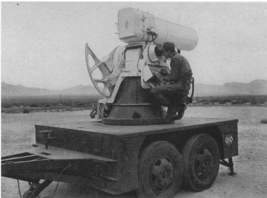
PIN-POINTING PLANES —This new Army Signal Corps optical tracker, developed at Fort Monmouth, N. J., can trace a moving plane 300 miles away in natural color on its scope through a powerful, 160-inch lens. The steerable instrument, weighing a ton and a half, is designed to operate with radar sets. Pvt. Lee Harsburger, Leipsic, Ohio, is operating the equipment.
