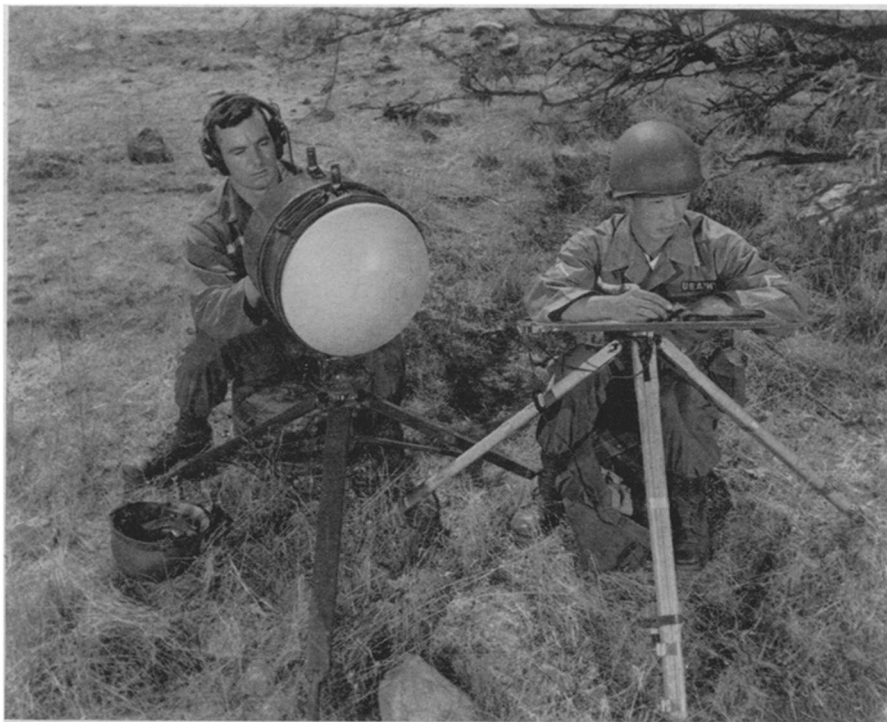
PORTABLE RADAR —The lightweight radar being operated here by Pvt. Thomas Hughes of Kearny, N. J., while Pfc. Thomas Yamada of Honolulu, T. H., plots the results, weighs only 85 pounds, compared to the ton or more of most Army radars. The midget radar set, built for the Army by Sperry Gyroscope Company, produces an audible signal when a man or object is within range instead of the usual visual signal, thus eliminating the cathode ray tube.
