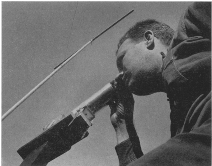
MOONWATCH TELESCOPE —A volunteer observer, Nelson M. Griggs of Washington, D. C., here demonstrates how the telescope especially developed for spotting an earth satellite can be used with a meridian marker.
