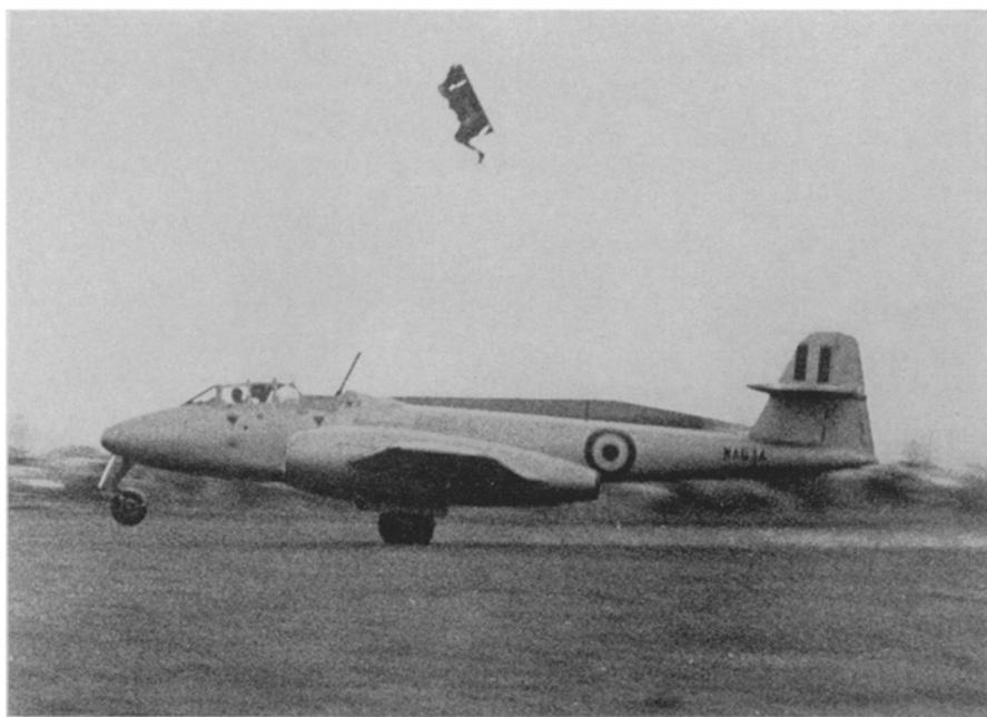
GROUND LEVEL BAIL-OUT —Royal Air Force squadron leader J. S. Fifield gave living proof of the ground-level efficiency of a British automatic ejector seat at Chalgrove Airfield, Oxfordshire, England, when he was hurled from a jet moving along the runway and floated safely to earth. He is shown here seated in the air before his parachute opened.
