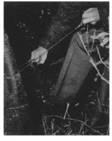
rings, attached to each end of the foot-anda half-long blade, as shown in the photograph. To saw, the tool is pulled back and forth. Folded, the saw fits into a pocket. Science News Letter, January 26, 1957
