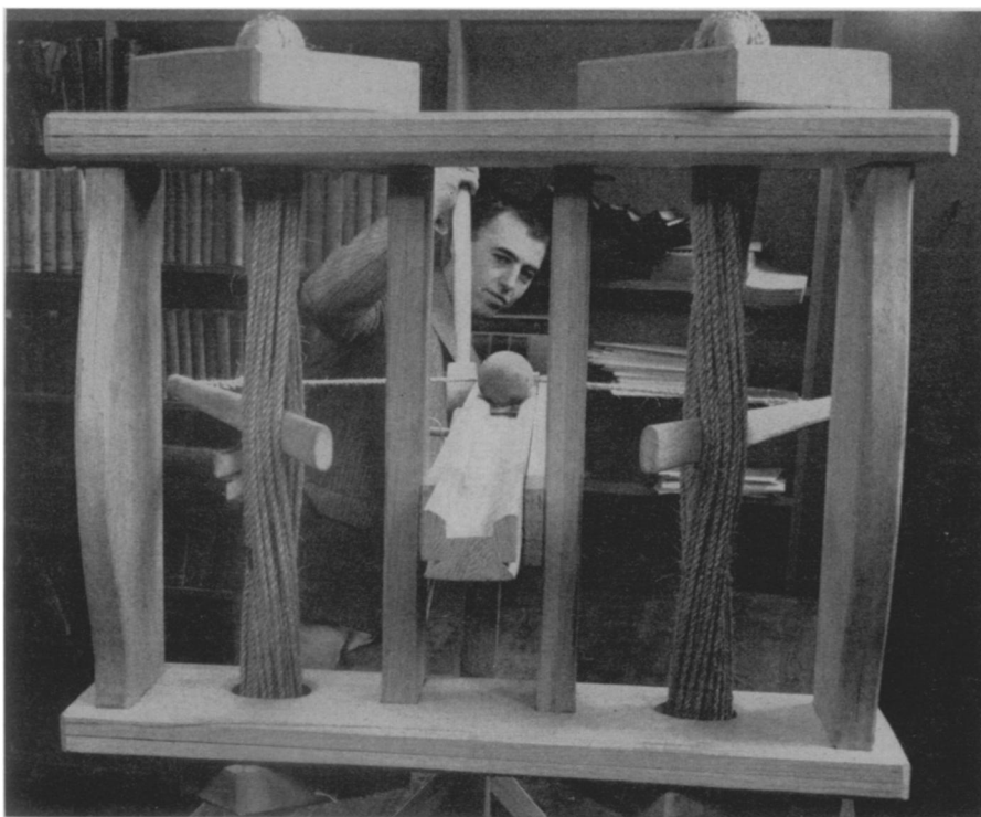
CATAPULTING INTO THE PAST —An exact replica of a catapult used in 200 B.C. was built by Richard G. Plummer of Milwaukee, Wis., a Cornell student. The catapult, invented by the Greeks and copied by the Romans, was standard artillery until about 300 A.D. Using a torsion principle of propulsion, it made a fundamental change in warfare. The strands of rope (the Greeks used animal gut or human hair) were twisted by drawing back bow-like arms inserted in them, and the projectile discharged by releasing a trigger.
