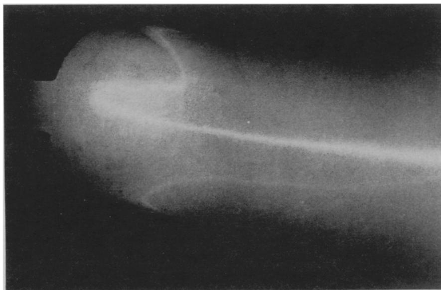
EARLY U. S. "PINCH EFFECT" —This photograph shows the "pinch" going around a curve in xenon gas in an early Perhapsatron torus, which is a doughnut-shaped apparatus, the Atomic Energy Commission explains.
