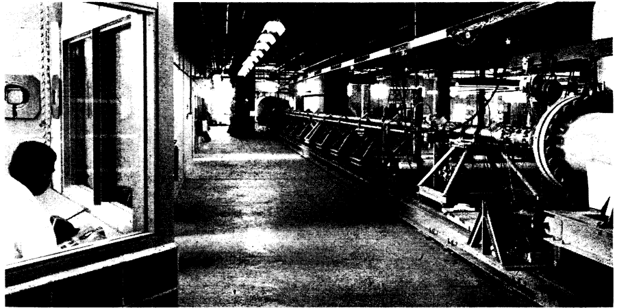
HYPERSONIC SHOCK TUBE —From the control room a technician can unleash speeds of 18,000 miles per hour and temperatures of 15,000 degrees Fahrenheit in this 100-foot-long shock tube built by Avco Manufacturing Corporation, Everett, Mass.
