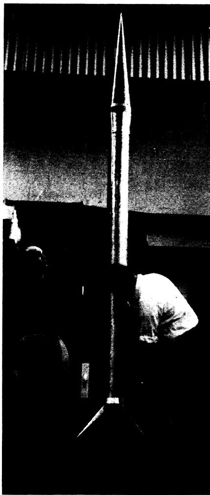
CAJUN ROCKET —This rocket is one of 16 that the University of Michigan will fire 75 miles into the air above Ft. Churchill, Canada, during the International Geophysical Year. It will use the propulsion unit from a Nike anti-aircraft missile. William Hansen and Theodore Pat- tinson examine the rocket.
