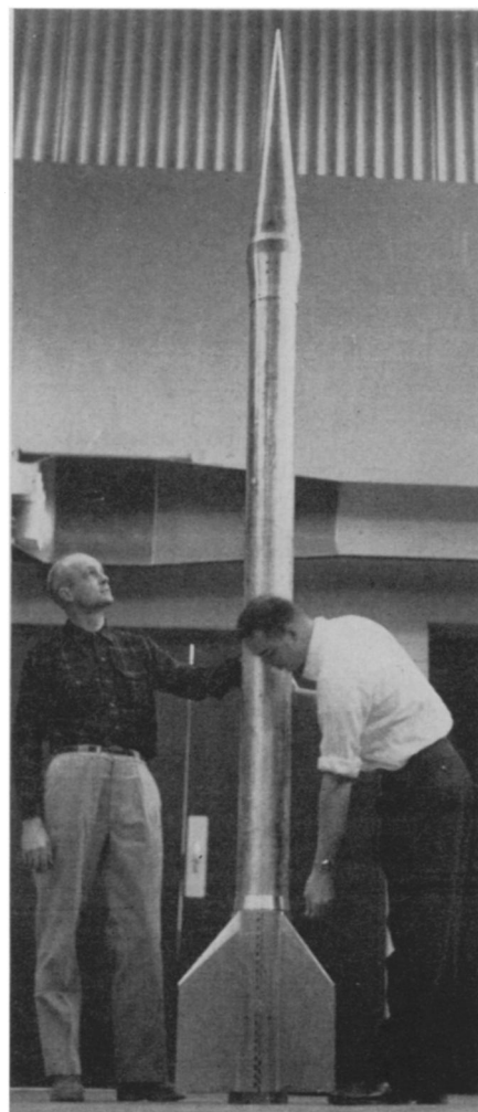
CAJUN ROCKET —This rocket is one of 16 that the University of Michigan will fire 75 miles into the air above Ft. Churchill, Canada, during the International Geophysical Year. It will use the propulsion unit from a Nike anti-aircraft missile. William Hansen and Theodore Patinson examine the rocket.
