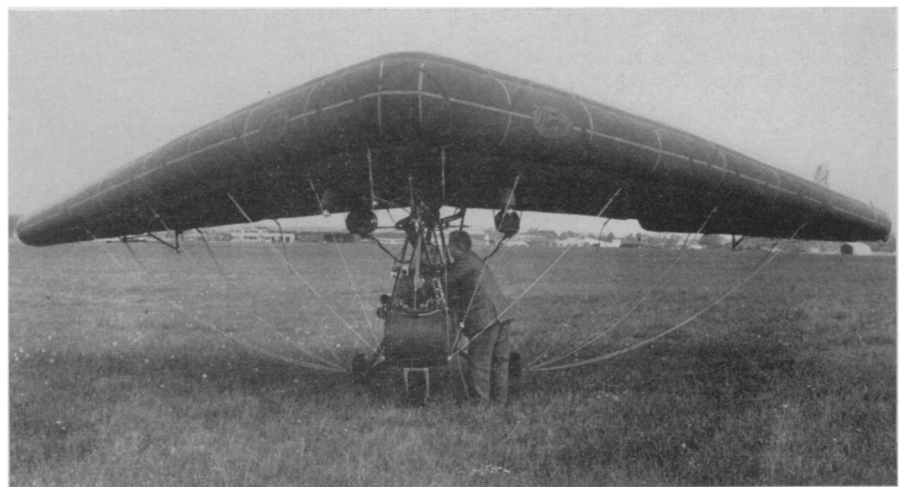
INFLATABLE AIRPLANE —Great Britain's newest airplane is blown up like a balloon. The wings of the ML Utility airplane are composed of a single delta-shaped inflated rubber fabric envelope, in which pressure is maintained to provide a stiff aerodynamic surface. The wings can be detached after use and rolled up into a bag. The aircraft can cruise at 50 miles per hour and its take-off run is only 90 yards.
