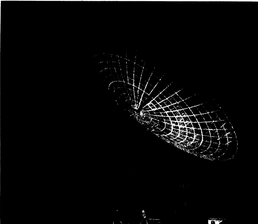
MOON BOUNCER —The Diana moon radar antenna, a development of the Army Signal Corps Engineering Laboratories, Fort Monmouth, N. J., is being used to calibrate equipment for the Minitrack stations in preparation for tracking the earth satellites. It "illuminates" the moon, which means the huge radar is hitting the moon with a very strong signal.
