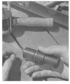
tor is housed in a two-part case molded of a butyrate plastic. The buzzer operates when the two halves of the case are screwed together.
