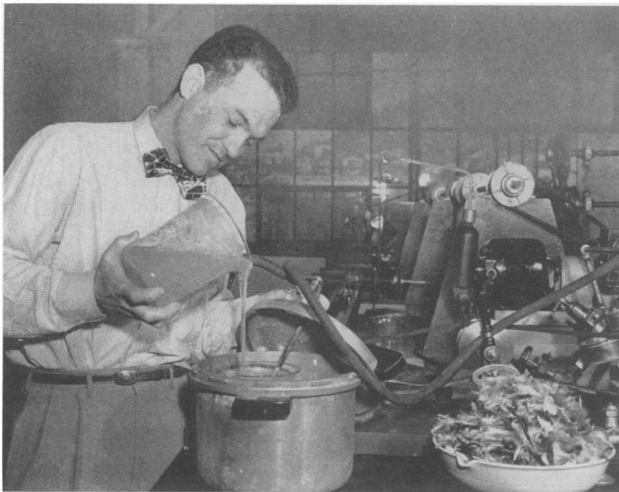
FABRIC FROM FEATHERS —The bowl on the right holds chicken feathers, destined to become fibers. R. A. O'Connell, of the U. S. Department of Agriculture, pours chemically treated poultry feathers, called "dope," into a pressure vessel. From the vessel the thick spinning dope will be forced through the tiny holes of a spinnerette and then given an acid-and-salt bath that sets the thin streams of dope into fibers.
