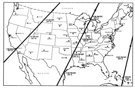
SATELLITE'S ORBIT—This map of the United States shows the predicted orbits of the Russian satellite sputnik for the dates Oct. 9 and Oct. 10. Between each pass, represented by the heavy black lines, the orbit shifts approximately 24 degrees west at the equator. Radio-tracking equipment and information supplied by the Mini-track stations provided the data used by the U.S. Naval Research Laboratory in compiling the map.
