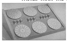
GENIAC, the first electrical brain construction kit, is equipped to play tic-tac-toe, cipher and encipher codes, convert from binary to decimal, reason in syl-
