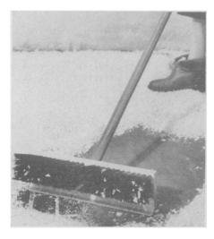
plastic. The brush, when turned over, has a steel blade for scraping and breaking ice. The brush-shovel combination weighs three and one-half pounds.
