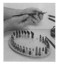
The threaded nibs, each of which holds a steel point, screw into the matching pen holder. The interchangeable, butyrate plastic nibs are available in different colors.
