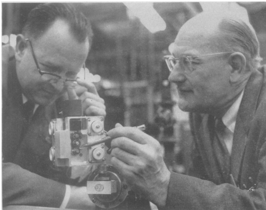
EXPLOSION SURVIVOR —Klystron oscillator, retrieved after a mid-air explosion in a long-range missile and a one and one-half mile free fall impact against the sea, is examined by Drs. Vincent E. Learned (left), Sperry Gyroscope Company director of klystron research, and Jack T. Muller, shock and vibration analyst for the company. The precision instrument was found to work "perfectly."
