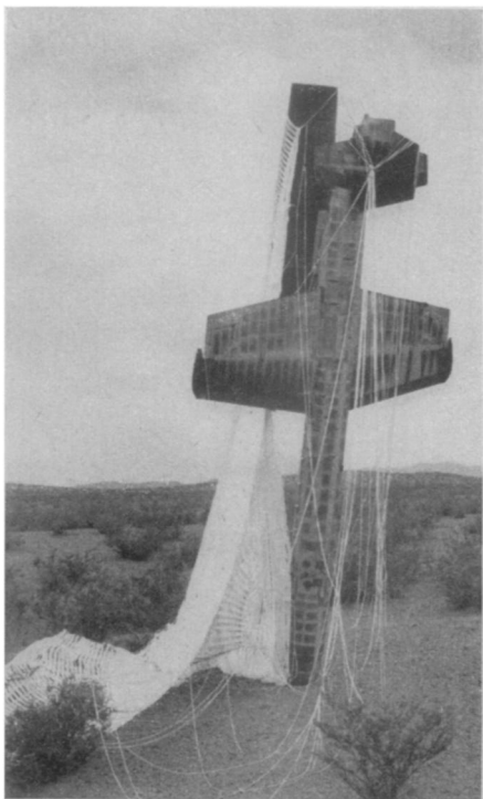
BURNED MISSILE — Air friction heat burned the black waffle pattern on the Lockheed X-7 ramjet missile that recently set new speed and altitude records. The parachute and nose spike enable it to be recovered and reflown.
