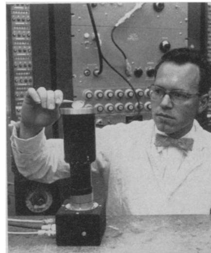
RADIATION ANALYZER —R. W. Perkins, General Electric chemist who developed the ultra-sensitive system of radiation analyses, places a small disc containing a river water salts sample on the probe portion of the electronic device.
