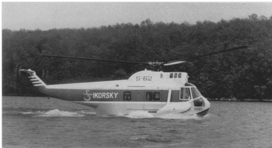
SEA COPTER —The new Sikorsky S-62 is believed to be the first amphibious helicopter ever built with a flying boat-type hull, suitable for operating from water, land, ice, snow or swamp. The hull weighs less than a land type hull equipped with inflated pontoons for water landings. Much of the drag associated with pontoon-type flotation, in flight and in the water, is also eliminated.
