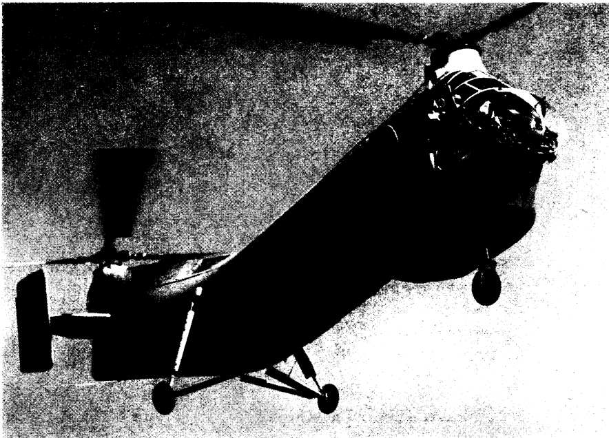
HANDS-OFF HELICOPTER —A helicopter is precisely stabilized during a "hands-off" flight (note pilot) as a result of an automatic flight control system developed by the Sperry Gyroscope Company, Great Neck, N. Y. Complete four-axis control, pitch, roll, heading and altitude, is provided in the system which takes its commands directly from the pilot's controls. Electronic trimming, automatic turn coordination and push-button controls for precise attitude adjustment are among the system's automatic features.
