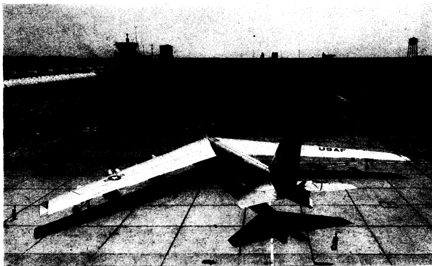
MISSILE PLATFORM —This new, long-range, eight-jet Boeing bomber will serve as a launching platform for supersonic, air-to-surface "Hound Dog" missiles. The aircraft is described as one of the U. S. Strategic Air Command's newest weapons; its increased range will allow the 450,000-pound Strato-fortress to span oceans and return to United States bases without refueling.
