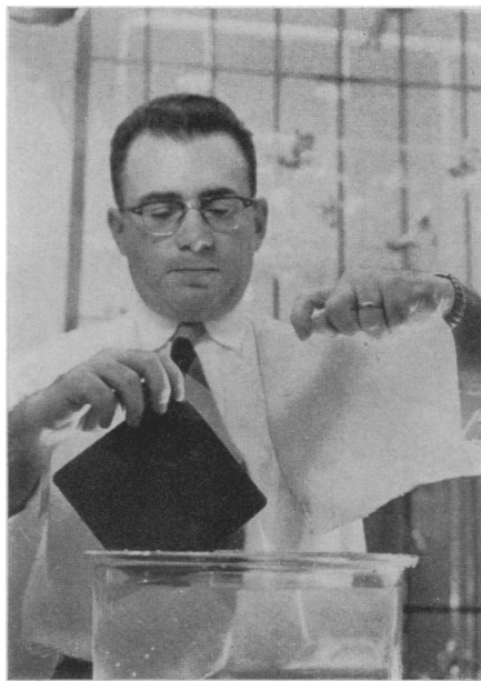
OIL RESISTANCE —Dr. Ben A. Bluestein of General Electric's silicone products department, Watertown, N. Y., shows how oil-resistant the new rubber (left) is compared with ordinary silicone rubber. Both samples were the same size before being placed in a jar of jet engine fuel.
