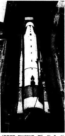
ADDED ENGINE—The U. S. Air Force's Atlas ballistic missile will have an intercontinental range of more than 6,000 miles as a result of the addition of a third engine. The new sustainer is in the center of the thrust section with booster engines on either side, as seen in this overhead view of the missile lying on its handling trailer. This view of the missile was taken as it was being backed into position for erection in the tower. Angled pipe above the center engine is the turbopump exhaust.
