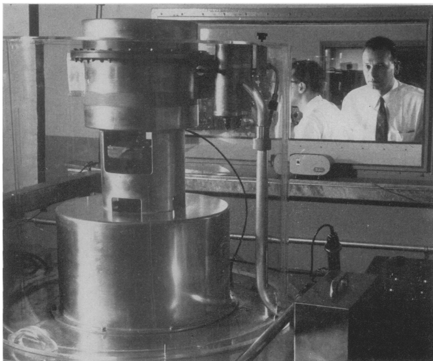
SPACE SHIP ENGINE —In a control room behind a protective glass wall Mr. Alfred Kunen (right) and associates at Republic Aviation Corp., Farmingdale, N. Y., run a test on the experimental apparatus of a "magnetic pinch plasma engine." In the high vacuum chamber (top, left), an electrical current, generated in the lower section, acts on a heavy gas and turns it into a plasma which is "pinched" and shot out of a nozzle outlet at very high velocities.
