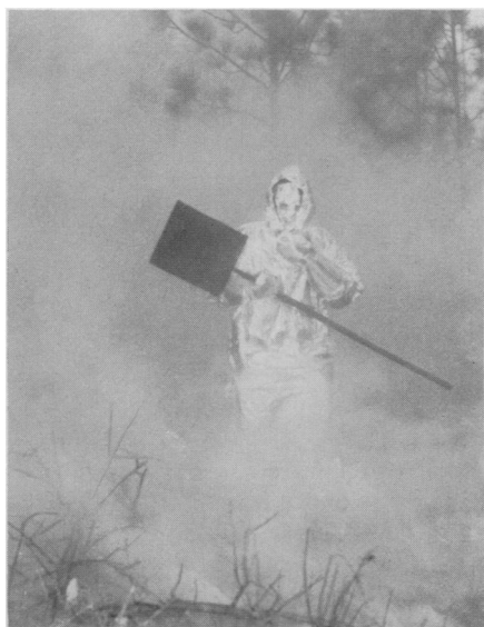
GHOSTLY FIRE FIGHTER —The U. S. Army's aluminum fire fighting suit, now undergoing intensive action tests, is made of flame-retardant, treated aluminized kraft paper laminated with a flame-resistant adhesive to a reflective aluminum foil. The face mask has tiny holes to give visibility.
