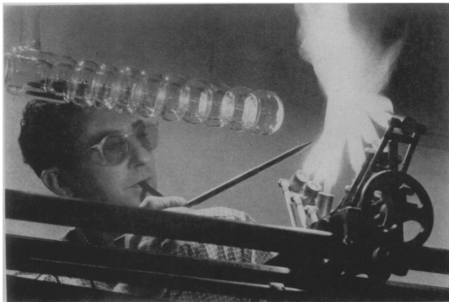
GLASS WORKER —An ancient art, glass blowing, is combined with modern technical skills to produce complicated scientific glassware. Earl Sexton, employed at the Indiana University chemistry department, works at a glass-turning lathe equipped with a multi-jet gas flame.
