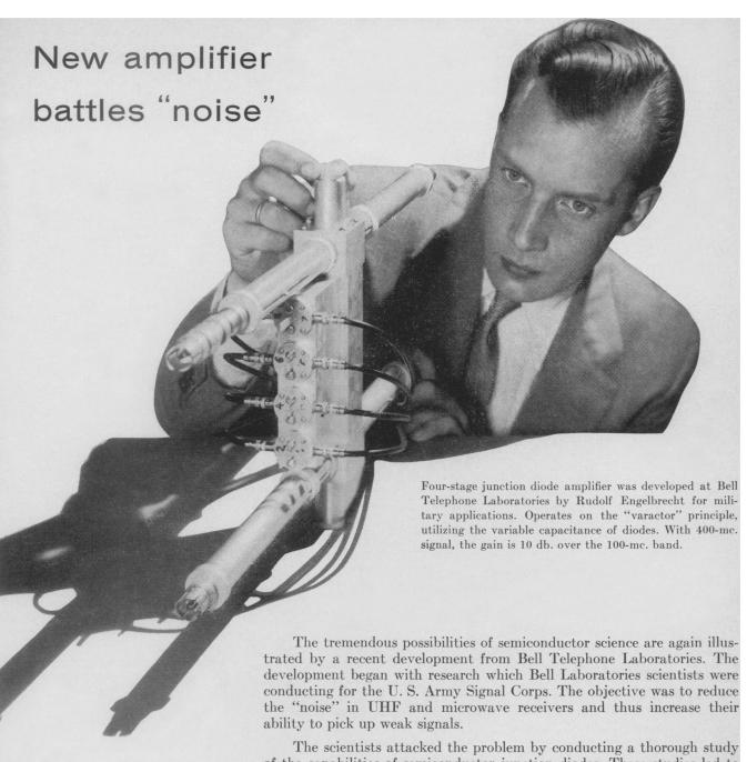
The scientists attacked the problem by conducting a thorough study of the capabilities of semiconductor junction diodes. These studies led to the conclusion that junction diodes could be made to amplify efficiently at UHF and microwave frequencies. This was something that had never been done before. The theory indicated that such an amplifier would be exceptionally free of noise.
