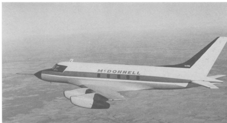
FOUR-ENGINE JET —The nation's first small four-engine jet airplane is designed to cruise at speeds of over 550 miles per hour. It has a normal range of 2,335 miles in still air with normal fuel reserves and was built by McDonnell Aircraft Corporation.
