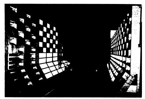
COAL CAR "LAMP OVEN"—Quartz infrared heat lamps have been used to thaw coal frozen in railroad hopper cars of the Western Maryland Railroad, operator of this test installation. This method may provide less maintenance, greater speed and economy, and less damage to railroad cars than in previous thawing methods. The infrared lamps were developed by General Electric in 1954. Fostoria Pressed Steel Company developed the oven.
