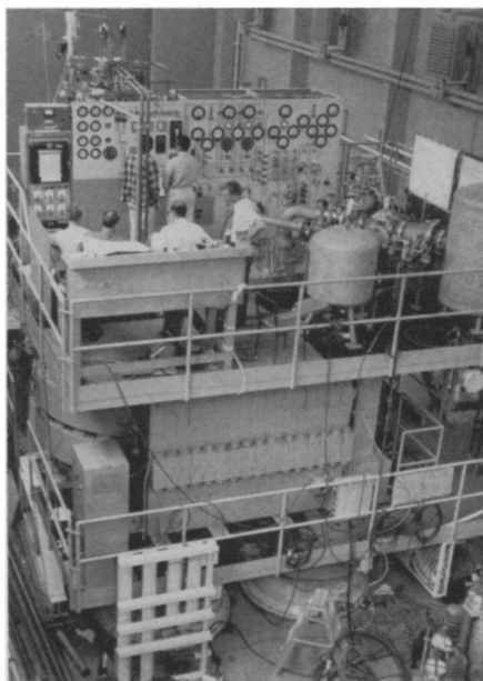
BUBBLE CHAMBER —The giant 72-inch "bubble chamber" in the University of California's Ernest O. Lawrence Radiation Laboratory, which is filled with liquid hydrogen, is used in studies of high energy nuclear particles generated by the Bevatron. The whole instrument weighs some 200 tons, and can "walk" by means of hydraulic "feet." The work with the instrument is a part of the fundamental research program of the laboratory sponsored by the Atomic Energy Commission.
